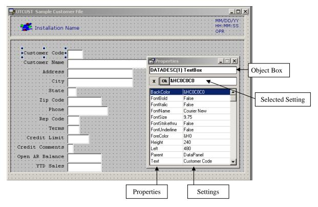
The attributes are a function of the object. The content of the box varies with the type of object. The Properties List is designed in a Visual Basic style.
