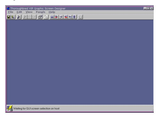
While this status message is displayed, another graphical screen or template can be selected for editing on the host using Dictionary-IV screen maintenance. This eliminates the need for the Graphic Screen Designer to be loaded each time a graphical screen or template is selected for editing.
