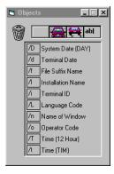
From the Object Toolbox you can drag and drop buttons, images, text, or any of the listed Dictionary-IV special characters. Once added, you can use Object Properties to set the attributes of the objects (see Object properties later in this manual).
