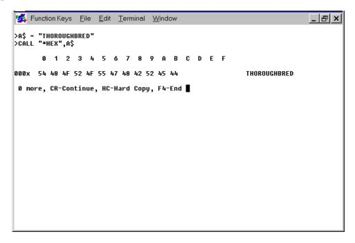
The \*HEX utility produced a hexadecimal dump to display contents of the A\$ string variable. The message line at the bottom of the listing displays a set of options that will prove useful when you have a very long string contained in a string variable.
