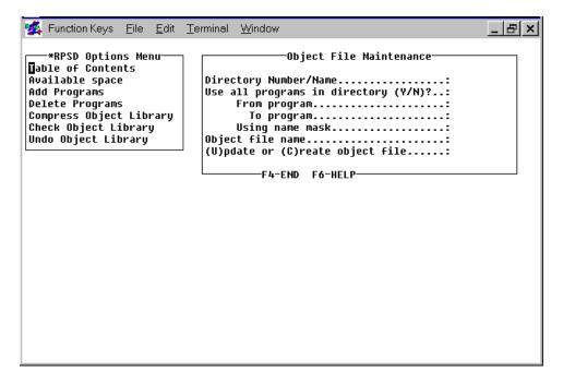
The screen contains two windows. You must select an option from the \*RPSD Options Menu and enter the required information in the Object File Maintenance window.
