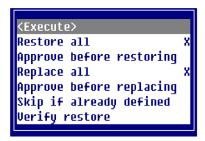
This selection allows you to select one restore rule and one replace rule. You also have the option to verify any combination of restore and replace rules selected. Once your selections are made highlight **Execute>** and press **Enter**. This will execute the restore with the specified/selected options.
