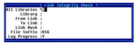
For the Links you want to check, select all libraries, a single library, and a range of Links with or without a mask, with or without a file suffix. Select Y to log the progress. Once the check is completed you can view the Link Integrity Log.
