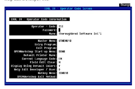
If an operator code is defined as a **Help Edit Developer** and the on-line help definition does not exist in the current language, the developer will have the ability to define the on-line help.
