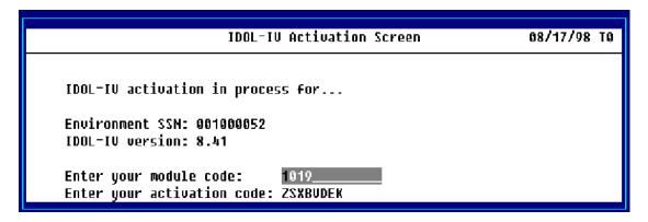
The system displays the Environment SSN and the Dictionary-IV version. You enter your module code and activation code.
