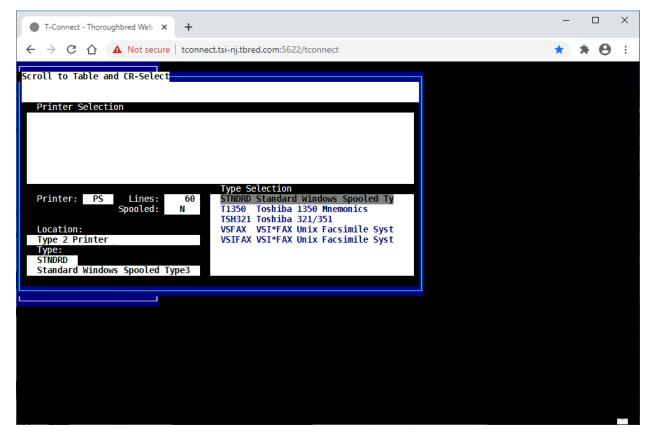
When a type 2 printer is selected as the output device, T-Connect will automatically generate the output in PDF format. Depending upon the browser settings, the PDF file will be downloaded and opened in a new tab, downloaded by the browser with an option to save the file, or the user will be prompted for an action. To change this behavior please refer to your browser settings.
