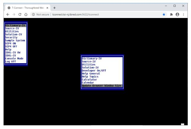
Another method to manually resize the terminal window is to print the Resize Window mnemonic, 'RW', in Basic console mode:
