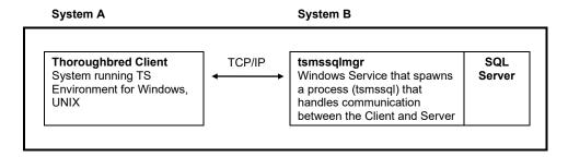
In the above figure the information is sent over the network to the server system. Once the requests reach the Server Process it creates SQL statements that are interpreted by the server system. The results are then passed back to the client through the Server Process.
